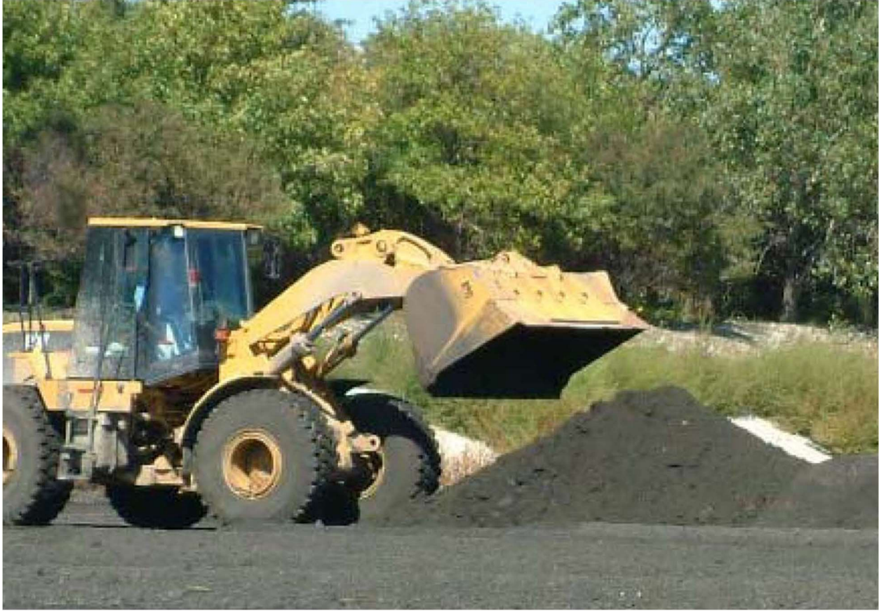
Exhibit 6. After about six weeks the wet biosolids have been air-dried sufficiently to be scraped off the paved drying area and stockpiled for loading into diesel-driven trucks for delivery to the ultimate disposal or utilization sites. Photograph courtesy of the MWRD.
