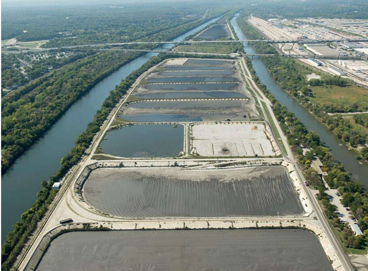
Exhibit 8. Aerial view of the sludge lagoons, foreground, and drying areas, center, looking southwest from above the McCook Reservoir. The Chicago Sanitary & Ship Canal is at left and the Des Plaines River at right. The MWRD railroad track runs along the left side of the lagoons and drying areas. Mannheim Road and the Illinois Tollway cross in the background. Photograph courtesy of the MWRD.
