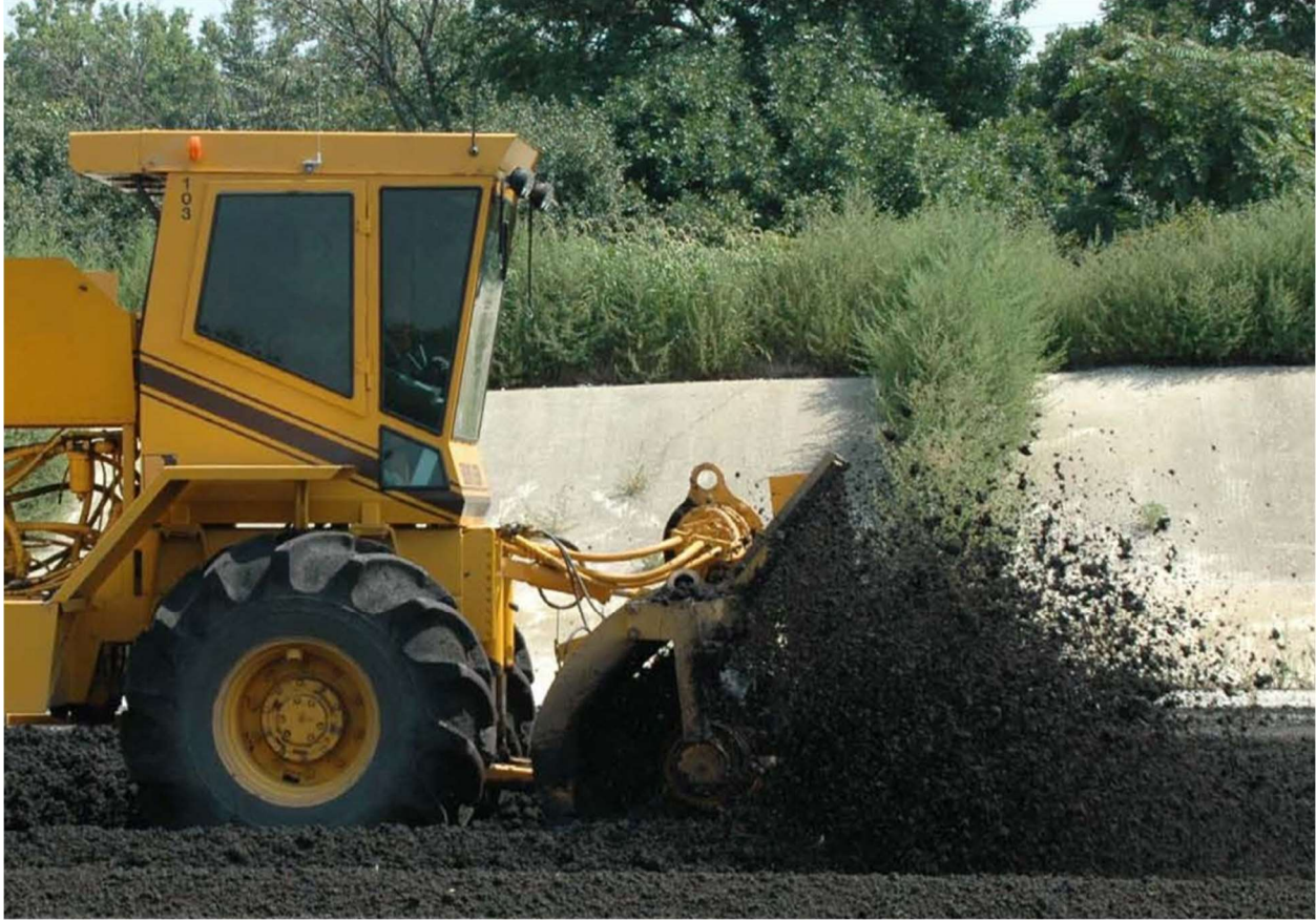
Exhibit 5. The second step in air-drying of centrifuge cake or lagoon sludge is breaking up the surface crust that forms from initial drying. Several passes over about six weeks are required to break up the surface crust and bring wetter sludge from below to the surface. Photograph courtesy of the MWRD.
