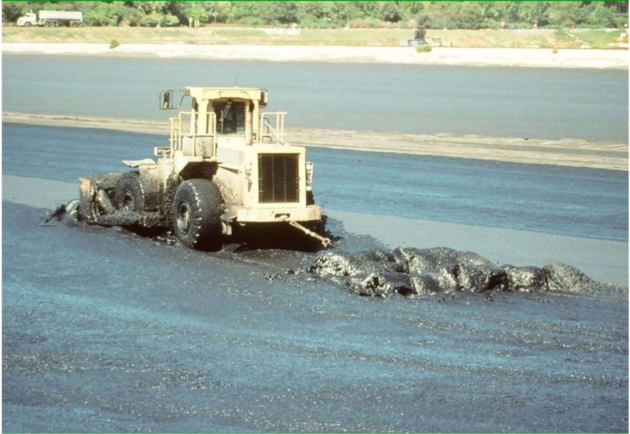
Exhibit 4. The first step in air-drying of centrifuge cake or lagoon sludge is spreading it out over the paved drying surface. Photograph courtesy of the MWRD.
